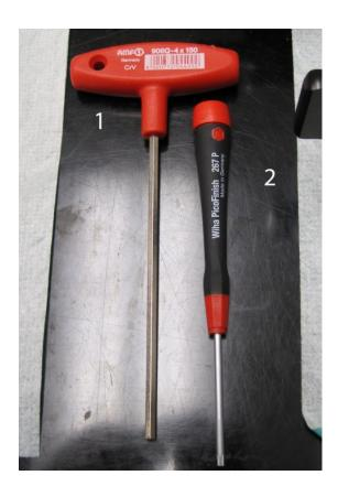
1: allen key- unscrews screw to remove or fasten ice tray
